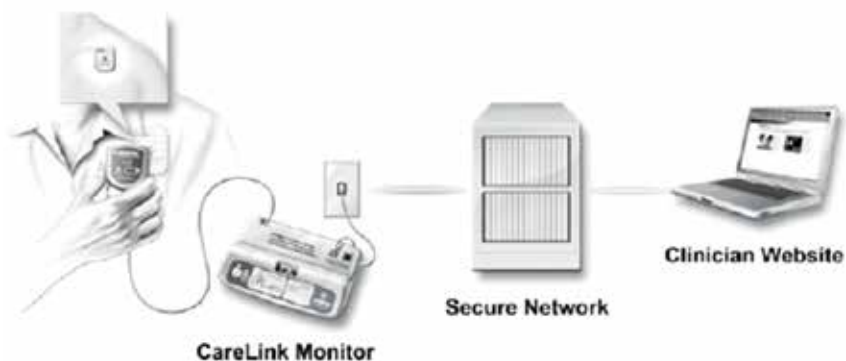
Figure 2. Remote monitoring system (Medtronic Carelink Network). Data from the pacemaker of ICD device is transmitted via the home monitor to a central secure network. Any abnormalities detected or problems with the device are relayed to the clinic, allowing them to be treated earlier.
